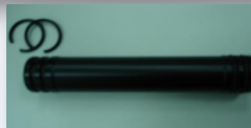
Cause broken o-ring
